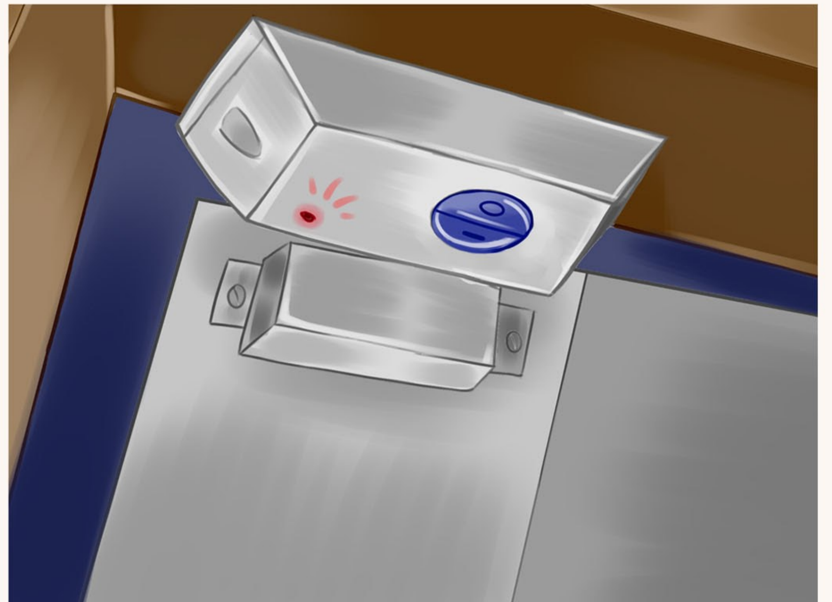
an alarm will be transmitted by the doorcontact
